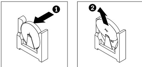
To remove the battery on the 5U server models with hot-swap power supplies (Model name: 2582-F4x), complete the following steps. For 4U server models with non-hot-swap power supplies, please see the above sub-section.
