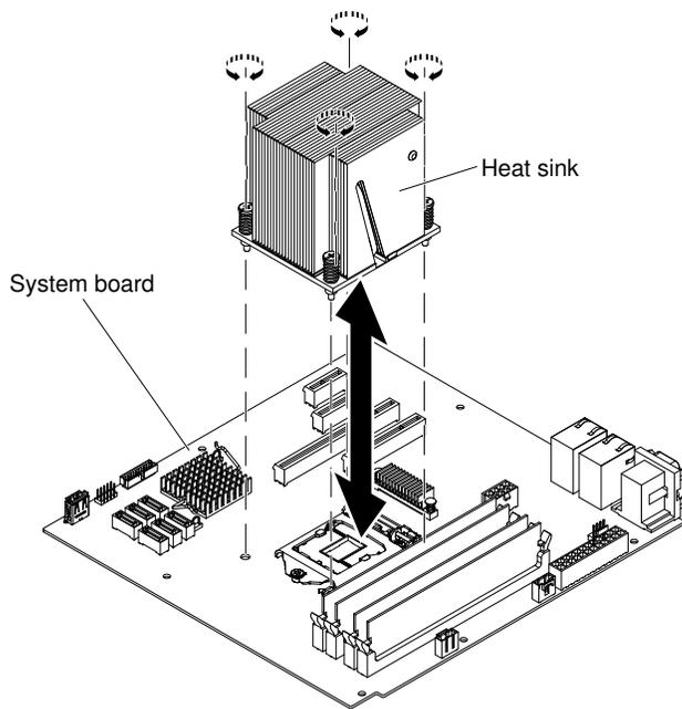
7. Reconnect any cables that you disconnected during the removal of the old microprocessor.
