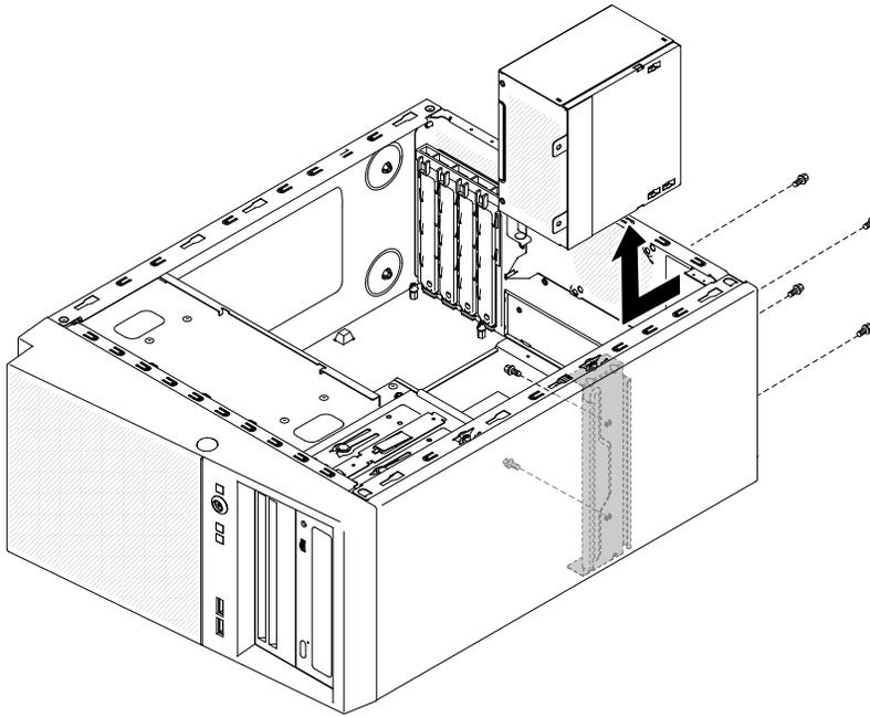
**Note:** You may find it easier to remove the power supply by pushing the bottom upward. Do not pull the cables.
