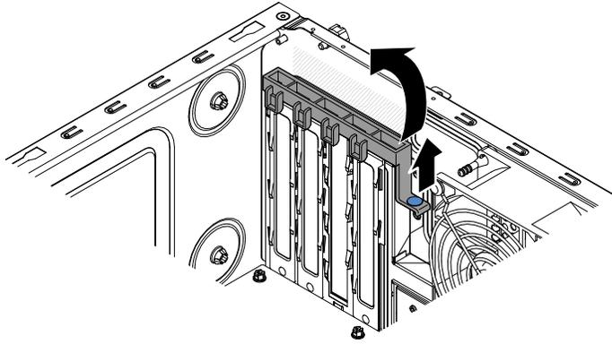
8. Rotate the rear adapter retention bracket upward to remove it from the chassis.
