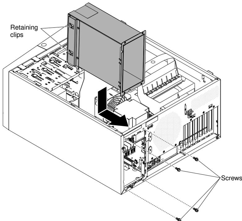
2. Install the other two screws to further secure the power-supply cage to the chassis, which is located in front of the power-supply cage.
