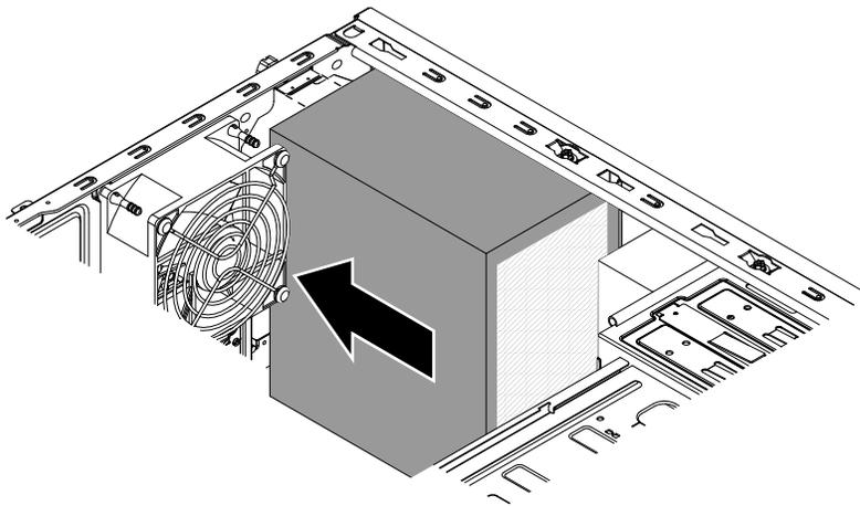
4. Install the screws that secure the power supply to the chassis.
