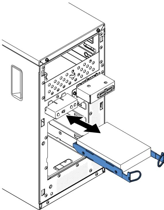
**Note:** Do not release the loops on the drive assembly until it is completely seated.
