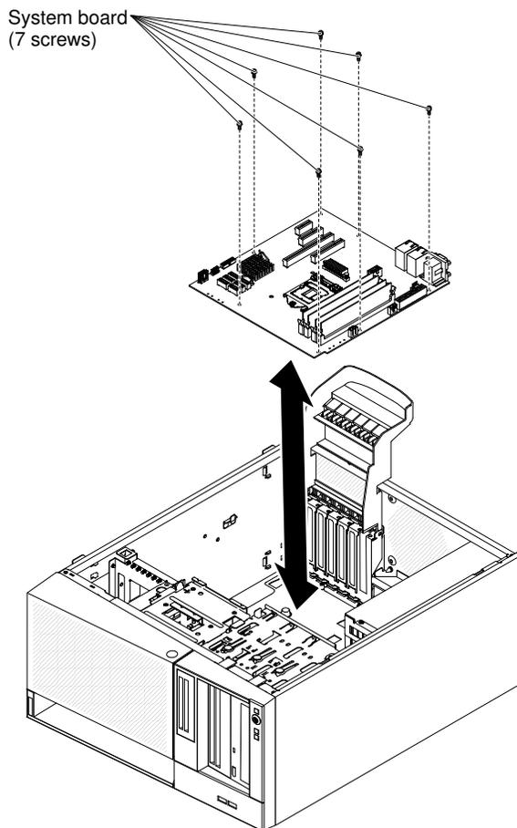
12. Carefully lift the system board out of the server.
