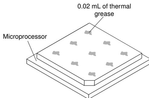
5. Use the thermal-grease syringe to place 9 uniformly spaced dots of 0.02 mL each on the top of the microprocessor. The outermost dots must be within approximately 5 mm of the edge of the microprocessor; this is to ensure uniform distribution of the grease.
