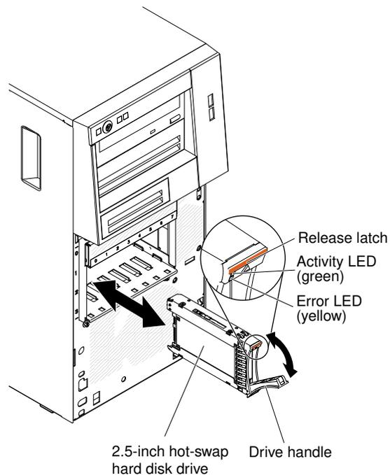
4. Grasp the handle of the drive assembly that is to be replaced and pull the assembly out of the bay.
