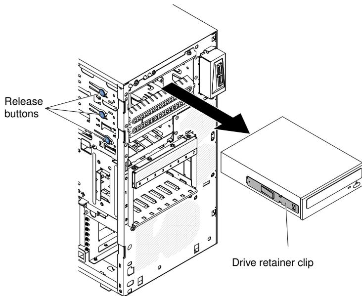
8. Remove the drive retainer clip from the side of the drive. Save the clip to use when you install the replacement drive.
