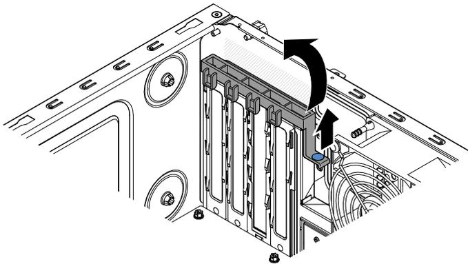
12. Rotate the rear adapter retention bracket upward to remove it from the chassis.
