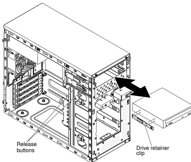
9. Remove the drive retainer clip from the side of the drive. Save the clip to use when you install the replacement drive.
