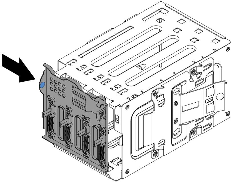
4. Slide the disk drive cage into the opening in the front of the server till half in.
