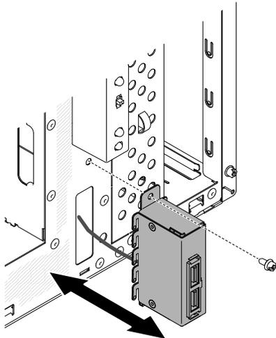
10. Carefully pull the front USB cable out of the opening in the chassis.
