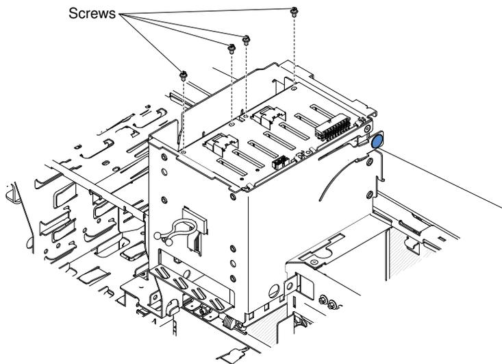
4. Press and hold the retaining tab on the side of the cage; then, rotate the drive cage into the chassis until it locks into place.
