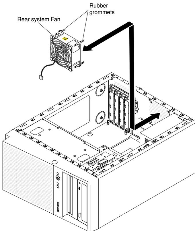
6. Connect the fan cable to the system board (see [“System-board internal connectors” on page 25](#) for the location of the rear fan connector).
