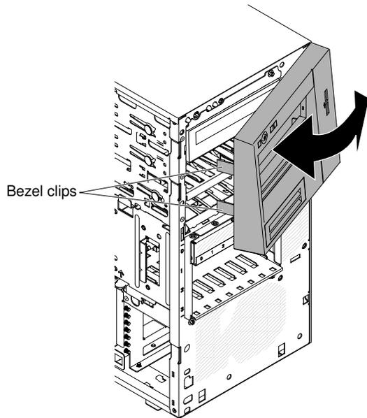
2. Rotate the upper bezel to the left side of the chassis until the bezel clips are aligned with the corresponding indentations on the left side of the chassis and snap them into place.
