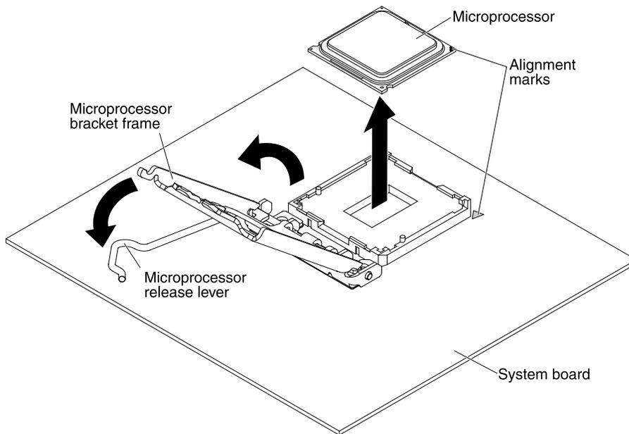
8. Open the microprocessor bracket frame by lifting up the tab on the top edge.
