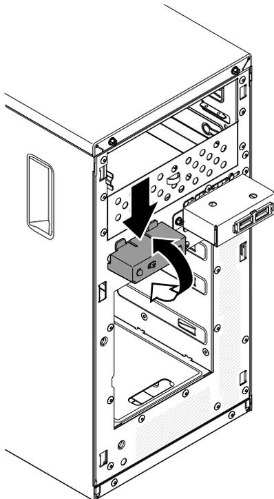
3. Push the front-panel assembly toward the chassis until it clicks into place.
