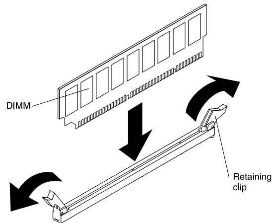
7. Touch the static-protective package that contains the DIMM to any unpainted metal surface on the server. Then, remove the new DIMM from the package.
