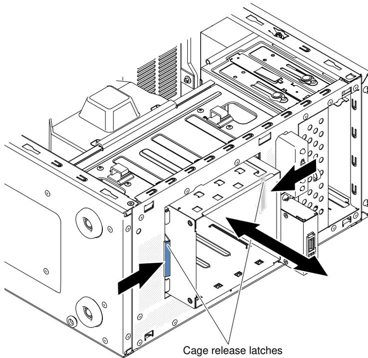
2. Align the bottom edge of the simple-swap backplate between the tabs and the bottom edge of the drive cage, and then rotate the simple-swap backplate toward the drive cage.
