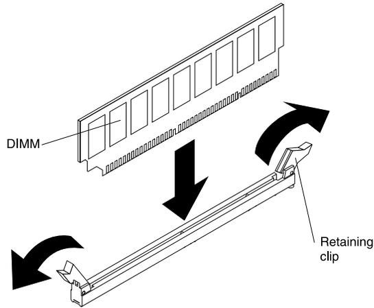
8. Touch the static-protective package that contains the DIMM to any unpainted metal surface on the outside of the server. Then, remove the DIMM from the package.
