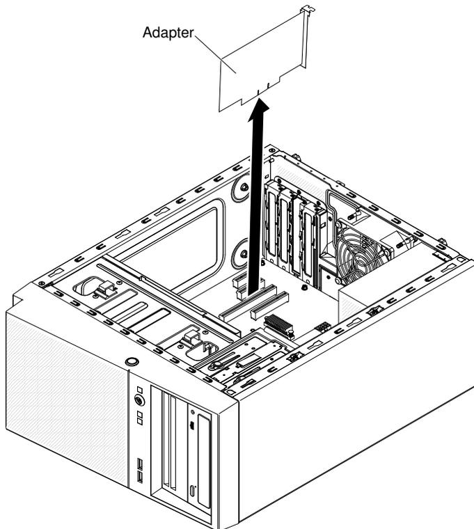
11. If you are not replacing the adapter, install an expansion-slot cover in the expansion-slot opening.
