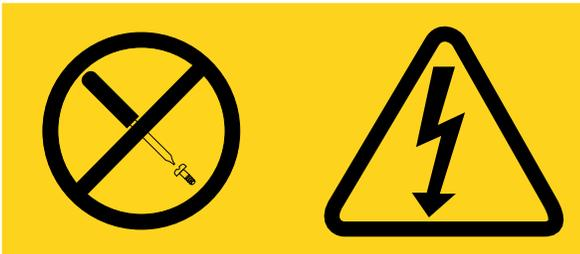
Hazardous voltage, current, and energy levels are present inside any component that has this label attached. There are no serviceable parts inside these components. If you suspect a with one of these parts, contact a service technician.
