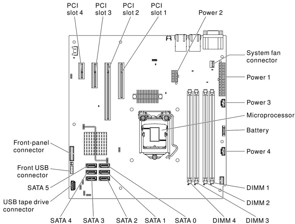
**Attention:** Static electricity that is released to internal server components when the server is powered on might cause the server to halt, which might result in the loss of data. To avoid this potential problem, always use an electrostatic-discharge wrist strap or other grounding system when you work inside the server with the power on.
