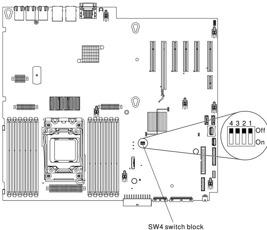
Figure 12. Power-on password switch
