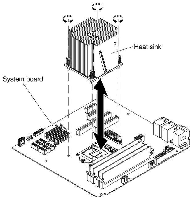
**Attention:** The microprocessor retention latch is spring-loaded when the microprocessor is in place. Releasing the latch too quickly or allowing it to spring upward can damage the microprocessor and surrounding components.
