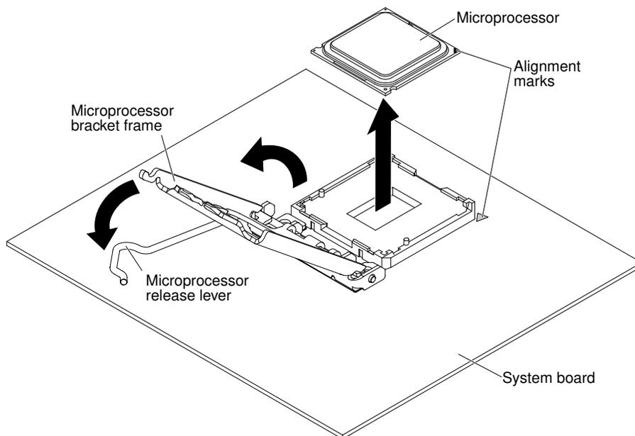
8. Open the microprocessor bracket frame by lifting up the tab on the top edge.
