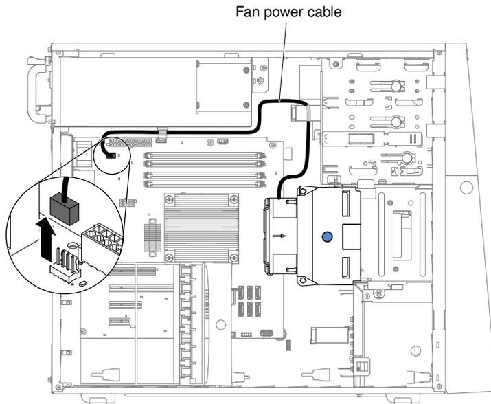
5. Grasp the hard disk drive fan duct by the blue point and pull up to lift it out of the chassis.
