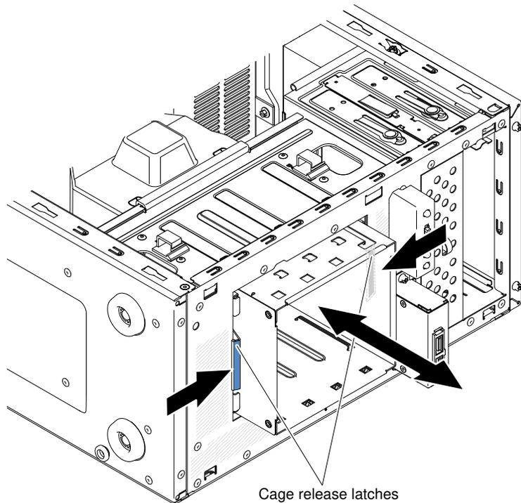
10. Carefully pull the hard disk drive cage and the cables out of the opening in the chassis.
