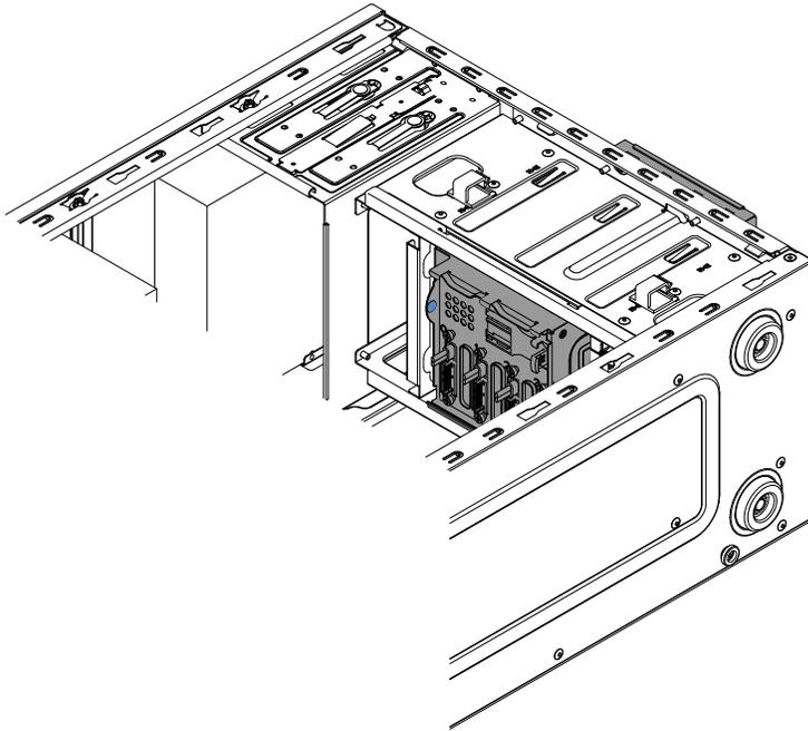
3. Touch the static-protective package that contains the system board to any unpainted metal surface on the server. Then, remove the system board from the package.
