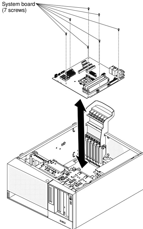
4. Install the seven screws that secure the system board to the chassis.
