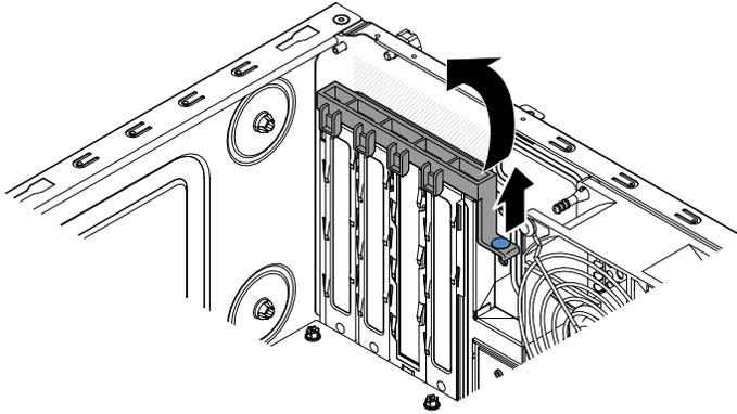
12. Rotate the rear adapter retention bracket upward to remove it from the chassis.
