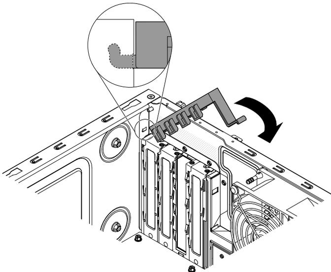
17. Rotate the rear adapter retention bracket into place so that the hole in the opposite hinge point snaps into place over the hinge pin on the chassis.
