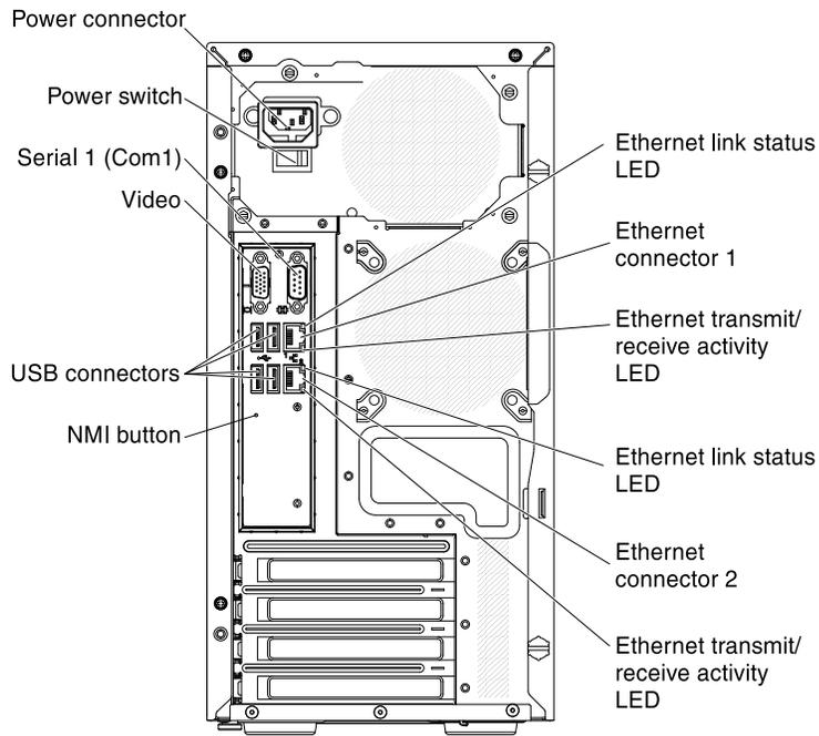
The following illustration shows the input/output (I/O) connectors on the rear of the 5U server model with hot-swap power supplies (Model name: 2582-F4x).
