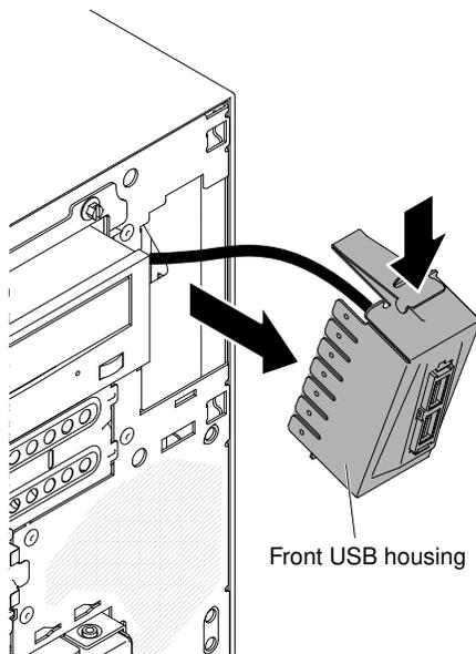
10. Squeeze the spring clips on the sides of the front USB connector assembly and pull the assembly out of the back of the housing.
