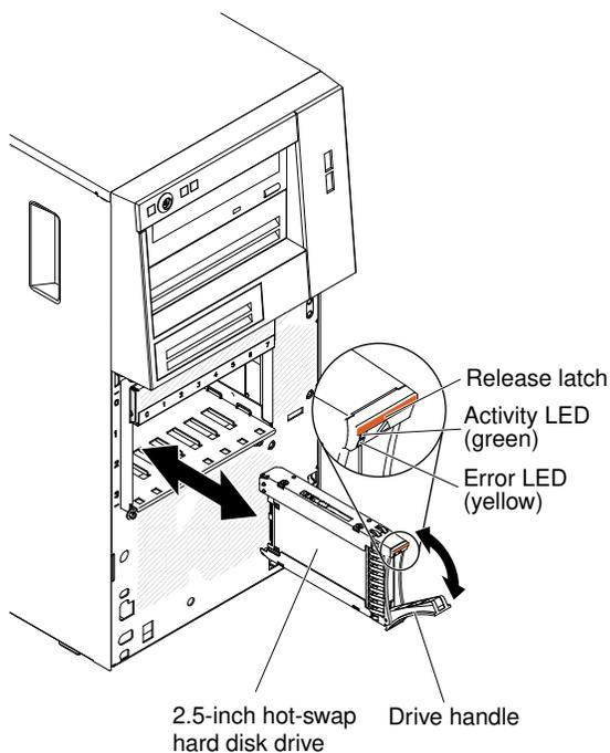
1. Touch the static-protective package that contains the drive to any unpainted metal surface on the server; then, remove the drive from the package and place it on a static-protective surface.
