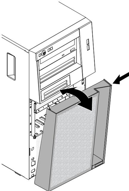
2. Rotate the top of the lower bezel up to the chassis; then, press the blue-colored release tab on the right side of the lower bezel and completely close the lower bezel until it locks securely into place.
