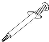
**Note:** If the grease is properly applied, approximately half of the grease will remain in the syringe.
