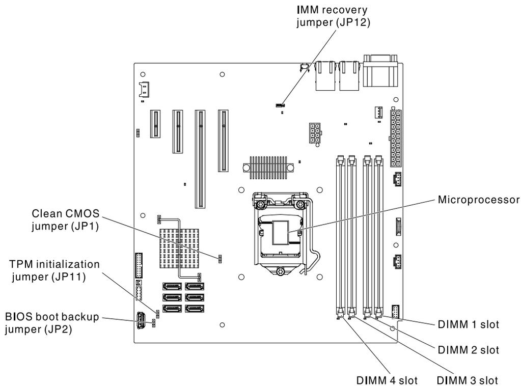
Figure 10. Location and description of switches and jumpers
