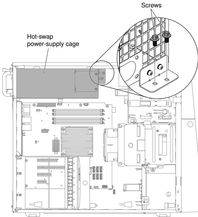
8. Remove the other four screws that also secure the power-supply cage to the chassis; then, slide the cage toward the front of the server to disengage the retaining clips from the top of the chassis and lift the cage out of the chassis.
