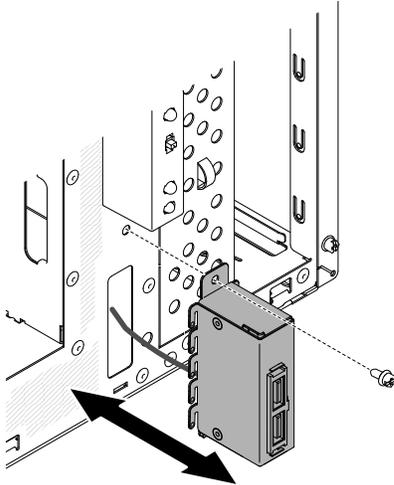
8. Place the tab on the bottom edge of the USB housing into the bottom of the opening in the chassis.
