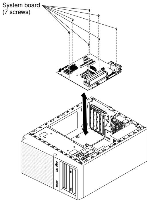
5. Install the seven screws that secure the system board to the chassis.
