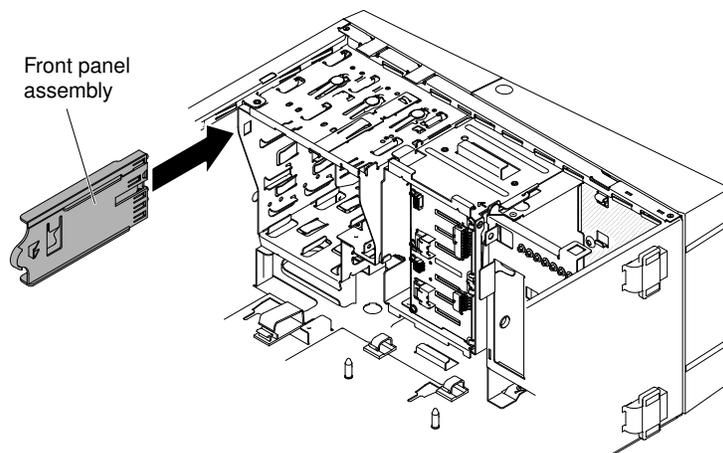
4. Reroute and connect the front-panel assembly cable to the system board (see [“System-board internal connectors” on page 25](#) for the location of the front-panel connector).
