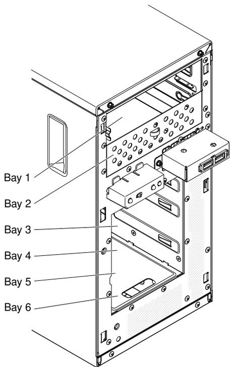
The following figure shows the locations of the drive bays in the 5U server model with hot-swap power supplies (Model name: 2582-F4x).
