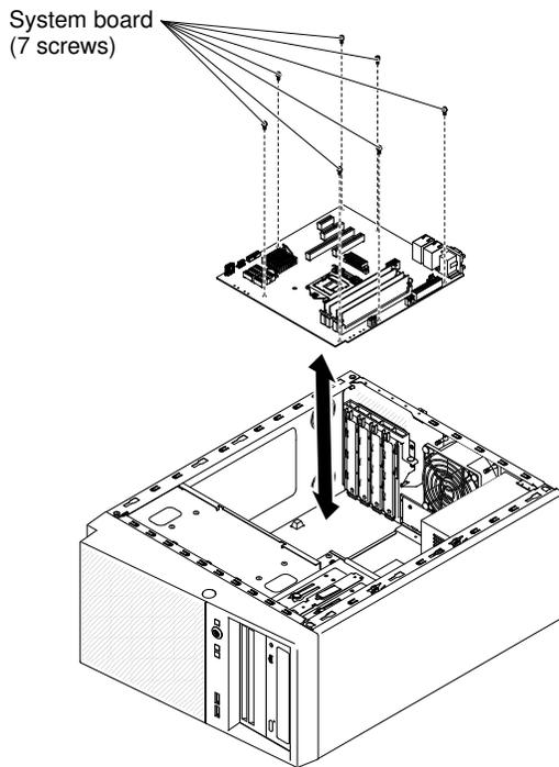
12. Carefully lift the system board out of the server.
