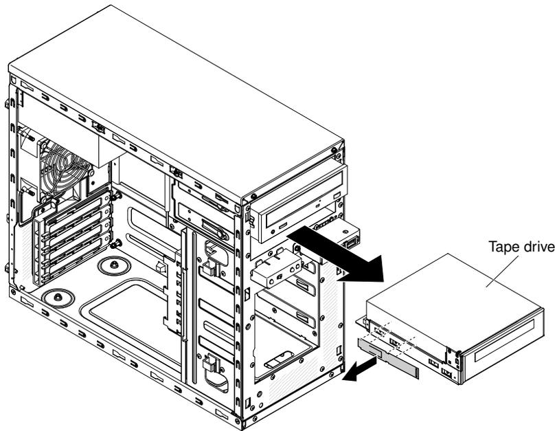
9. Remove the drive retainer clip from the side of the drive. Save the clip to use when you install the replacement drive.
