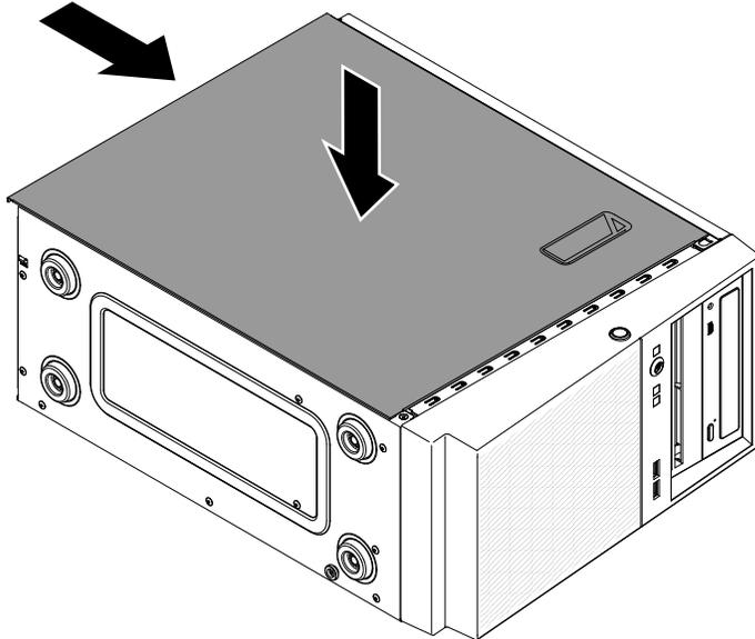
4. Secure the side cover in place with the two chassis screws on the rear of the side cover.
