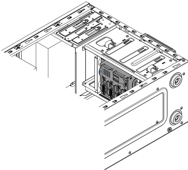
5. Connect the hard disk drive power cables to the backplate (connector P3 to bay 3, connector P4 to bay 4, connector P5 to bay 5, and connector P6 to bay 6,).
