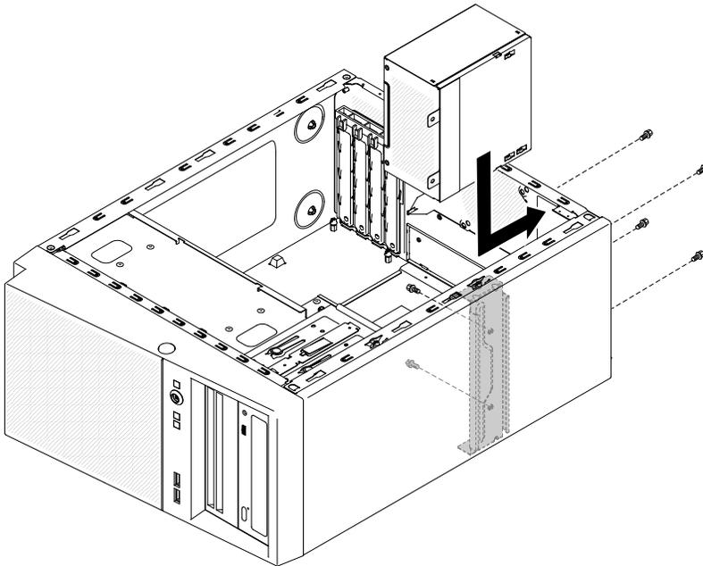
**Note:** Make sure the top and the bottom of the power supply align with the upper and lower tabs on the opening.
