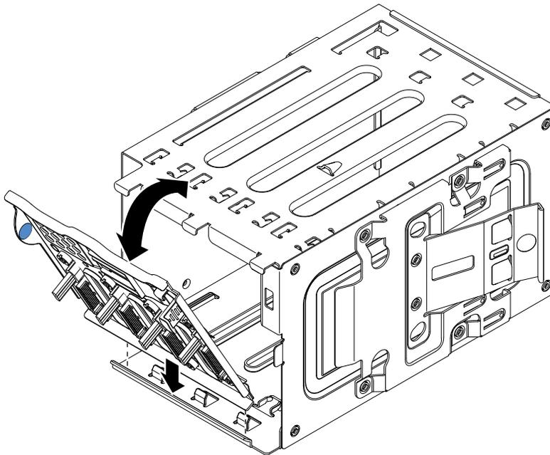
3. Make sure the tabs on the simple-swap backplate are on the left of the upper drive cage tabs, and then push the backplate till the end.
